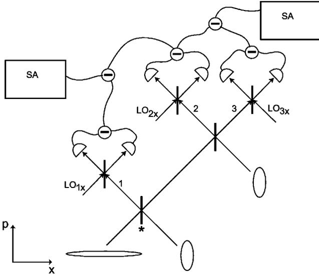
FIG. 1. Verification of genuine tripartite CV entanglement.  $x$  measurements: directly detecting the  $x$  quadratures of all three modes and electronically combining them in an appropriate way. The three-mode tripartite entangled state of modes 1, 2, and 3 in this figure is produced with three squeezers and two beam splitters (the star denotes a 1:2 BS).
