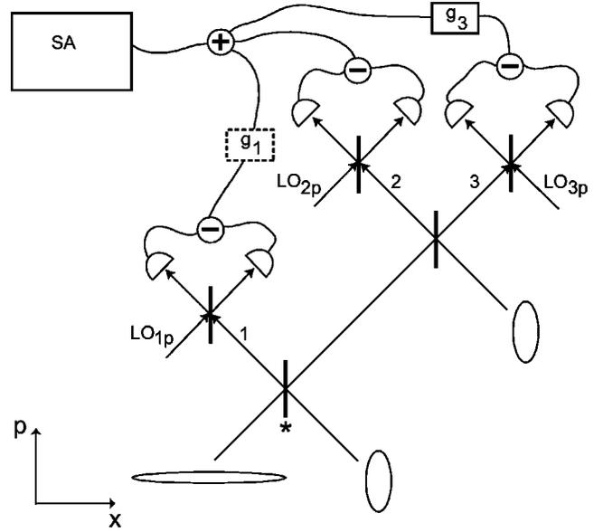
FIG. 2. Verification of genuine tripartite CV entanglement.  $p$  measurements: directly detecting the  $p$  quadratures of all three modes and electronically combining them in an appropriate way. The three-mode tripartite entangled state of modes 1, 2, and 3 in this figure is produced with three squeezers and two beam splitters. The parameters  $g_i$  are the “gains” from the conditions in Eq. (37) which can be chosen optimally (see the text later).
